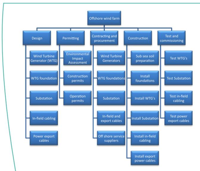
Figure 2.1 - Example Work Breakdown Structure
