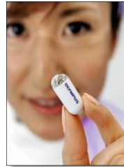
Camera pill with camera, transmitter and computer
